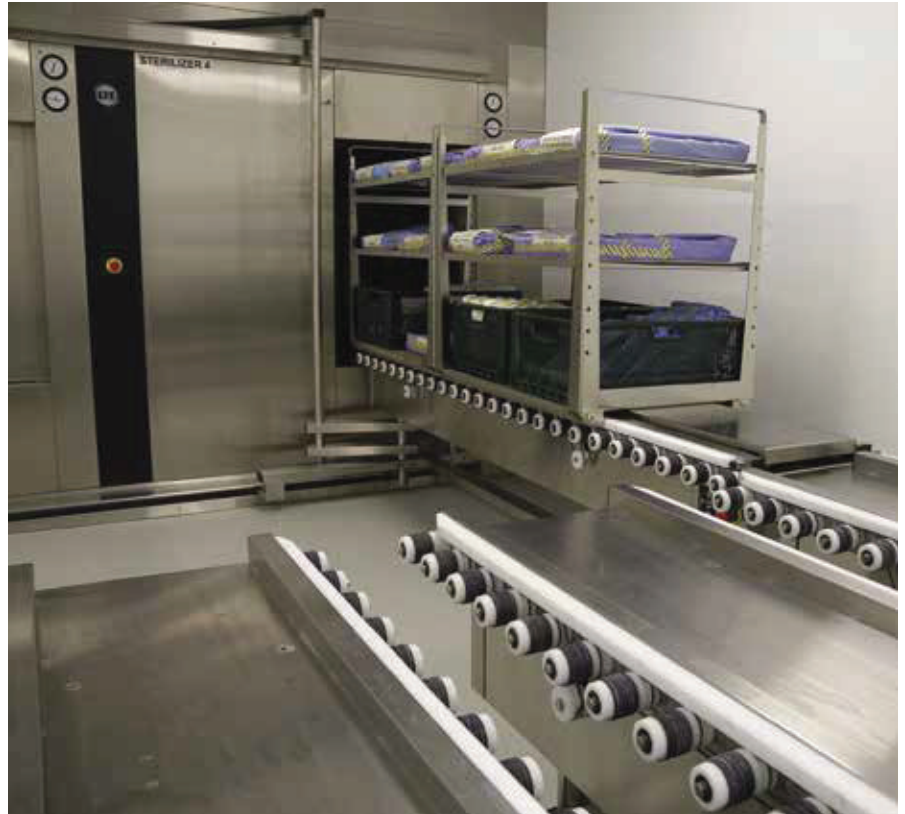
A processed load leaves a steriliser on the Remeda automatic unloading system
